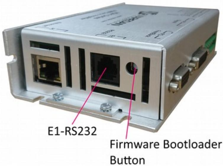
3. Connect the RJ12 serial cable as shown above to the E1 RS232 port.
